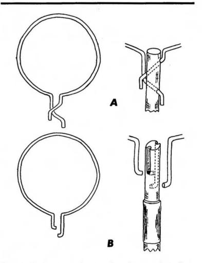
Figure 7. Net bag construction; two alternative ways of attaching hoop to handle.
