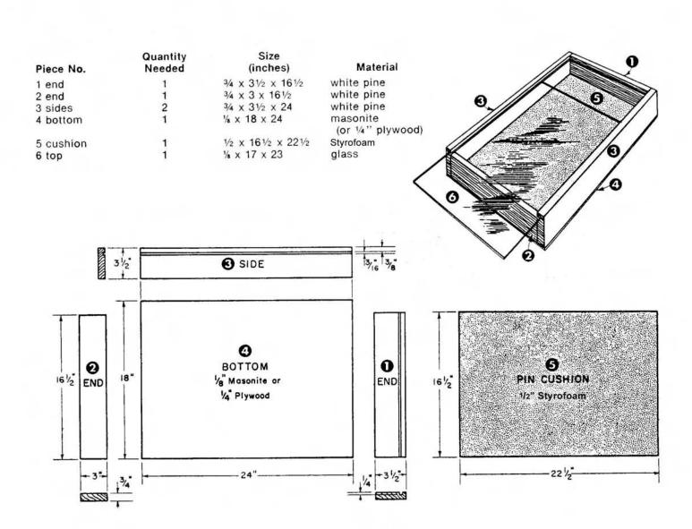
Figure 18. Insect display box and materials needed for its construction.
