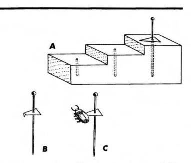
Figure 16. Pointing an insect: (A) setting height of point on pin, (B) tip of point bent down, and (C) insect correctly mounted on point.
