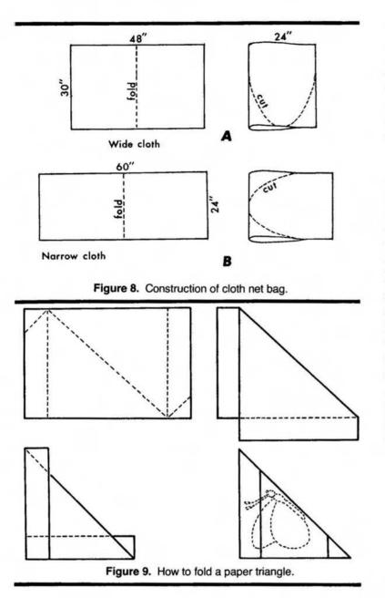
long as the diameter of the metal hoop. For example, if the diameter of the hoop is 15 inches, then the dimensions of the cloth should be as shown in figure 8. Cut the cloth to shape and pin the cut edges together to hold them while you sew. Fasten the open end of the bag to the wire loop by folding it over the wire and sewing with heavy thread.
