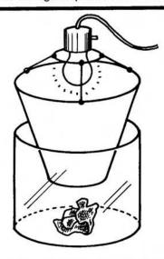
Figure 12. Alternate light trap with funnel.
