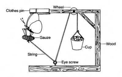
Figure 14. Weight lifting apparatus for testing the strength of insects.
