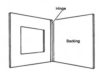
Figure 12. Hinging the mat to the backing.
