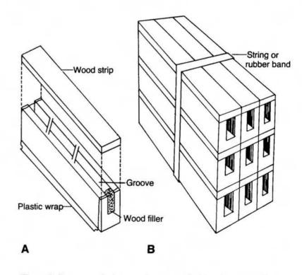
Figure 8. Trap nests for bees and wasps: a) individual trap nest, b) nine trap nests bundled together for placement in the field.
